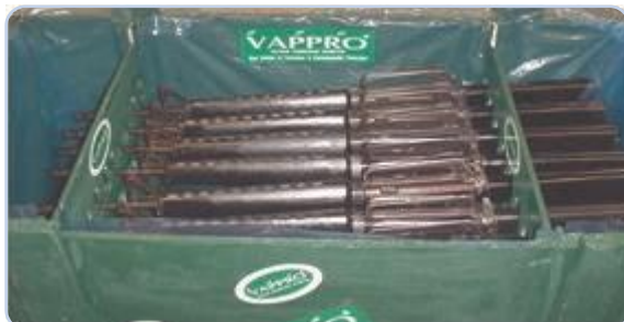
Cleaning and preservation of M16s using Vapro VBCI-818 CLP.
