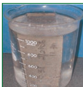
After 1500 hours Mild steel immersed in sea water with 700ppm of Vapro VBCI-844L
