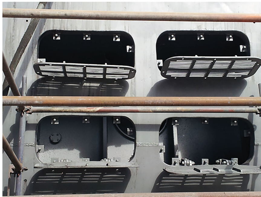
Figure 3. Ship opening, fitted with screens, for ballast water intake and discharge.
