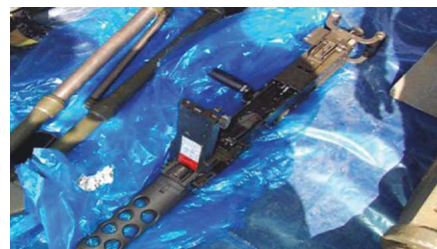
FIGURE 3 Weapon parts wrapped with transparent plastic sheets containing a VCI.
