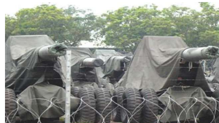
FIGURE 1 Heavy cannons on wheels covered with rough canvas fabric impregnated with a VCI.
