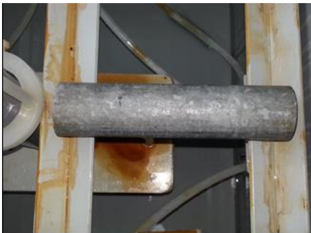
Picture (6) after 48 hours in the salt spray chamber.
