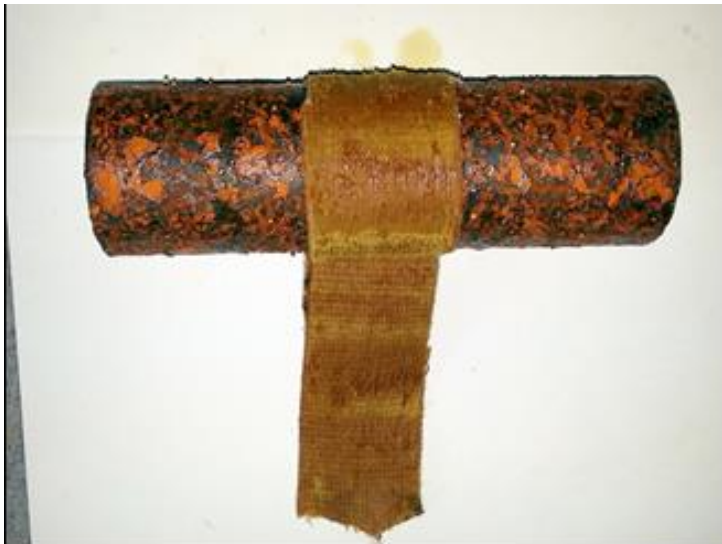
Picture (14) Vapro VCI Corro-Tape was unwrapped for observation
