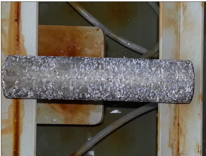
Picture (10) after 500 hours in the salt spray chamber.
