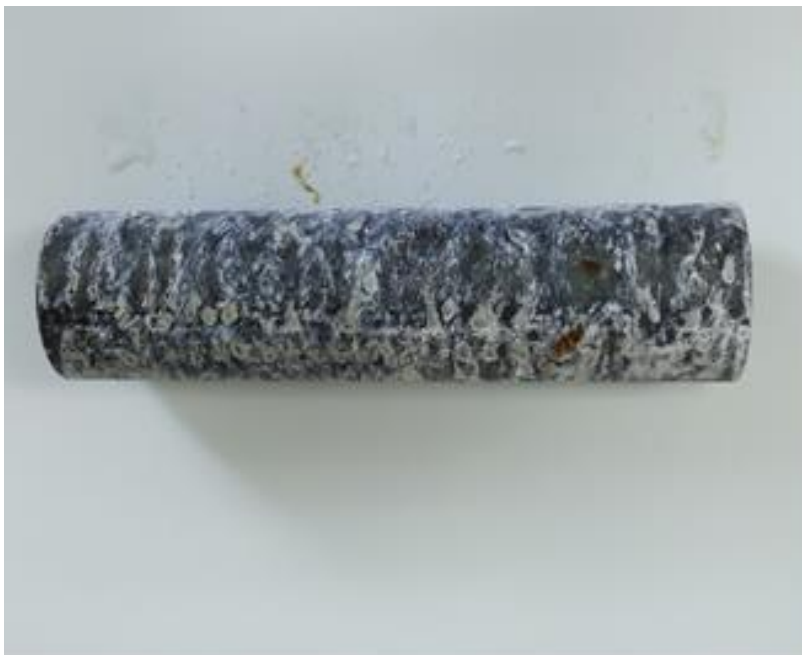
Picture (12) after 1000 hours in the salt spray chamber.
