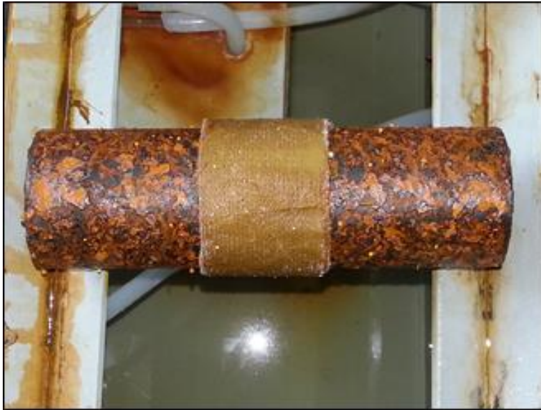
Picture (13) after 1000 hours in the salt spray chamber
