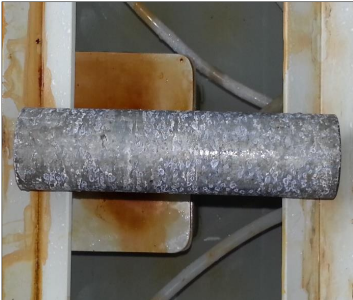
Picture (8) after 100 hours in the salt spray chamber.
