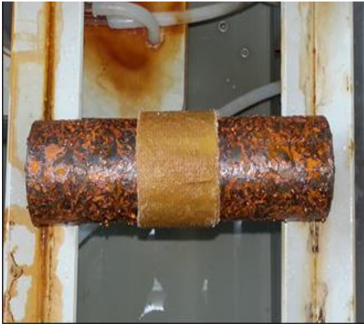
Picture (11`) after 500 hours in the salt spray chamber.
