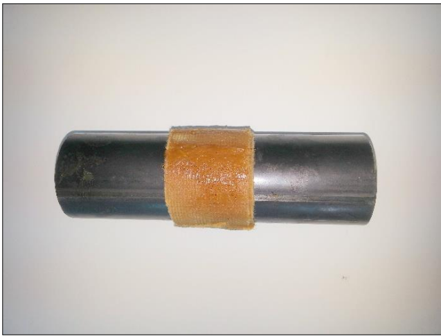
Picture (5) High Carbon Steel Pipe wrapped with Vapro VBCI Corro-Tape.
