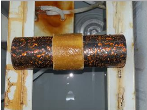
Picture (7) after 48 hours in the salt spray chamber.
