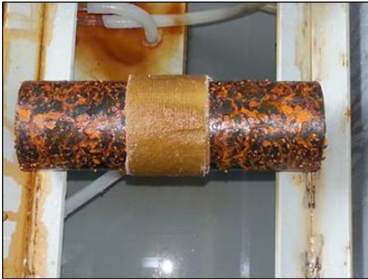
Picture (9) after 100 hours in the salt spray chamber
