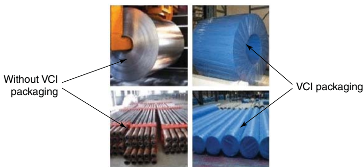
Figure 14.5 Pipes covered with VPCI packaging and uncovered. Source: Reproduced with permission from Gangopadhyay and Mahanwar [33]. Copyright 2018, Springer Nature.
