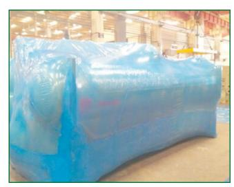
It thus enables effective and long term protection of ferrous and non-ferrous metals against corrosion /oxidation and tarnishing under adverse conditions including contaminants in air such as hydrogen sulphide, sulphur dioxide, ammonia or acid rain. Vappro VBCI vapors easily migrate to hard to reach areas like drilled holes, crevices etc. and give effective protection.
