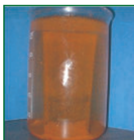
After 1500 hours Mild steel immersed in sea water without Vapro VBCI-844
